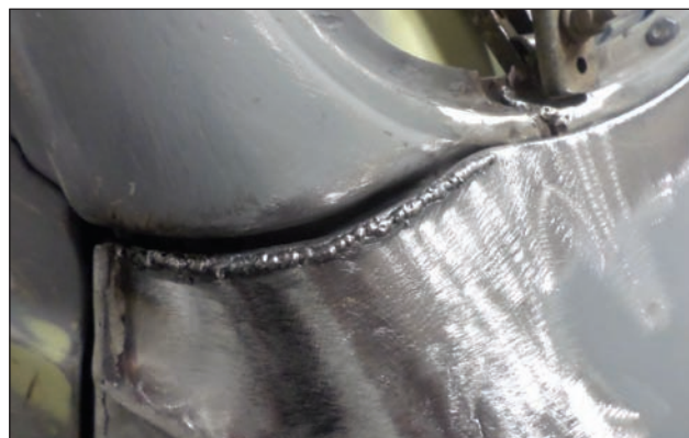
The top part of the cowl by the pillars needed help too. To close that gap, they first cut the cowl with a cut-off wheel and lifted the remaining metal up. Then they filled in that gap with weld as shown. (Photo Courtesy Lonnie Thompson)
