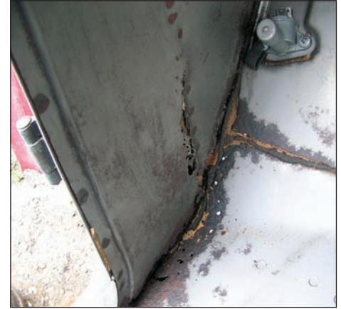
The inner kick panels usually see rust too. In this case, it's not that bad and can be repaired with some home-made patch panels. (Photo Courtesy Lonnie Thompson)
