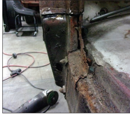
The rockers are always an obvious problem (this goes for most projects, regardless of make), but once you cut away the outer panel, you can see the real problem: the inner rockers. If the outers are gone, the inners probably are too. (Photo Courtesy Lonnie Thompson)
