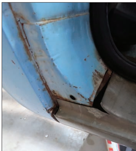
Sometimes you'll run into another problem: poorly fixed panels. In this case, the panel probably got water in the gap, so replacing it makes sense. (Photo Courtesy Lonnie Thompson)
