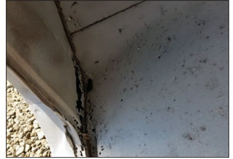
See the rust here and those little pits? Those are some small to large amounts of rust that the media blasting process removed that will need to be replaced. (Photo Courtesy Lonnie Thompson)
