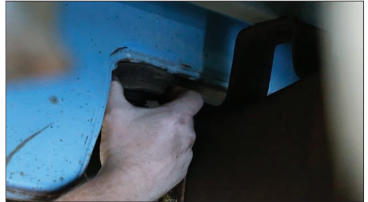
Removing the old cab mounts is pretty simple: unbolt them, jack up the side of the truck, and then lift them out. If you're concerned about damaging the rockers, use a block of wood between the jack and the panel to distribute the load.
