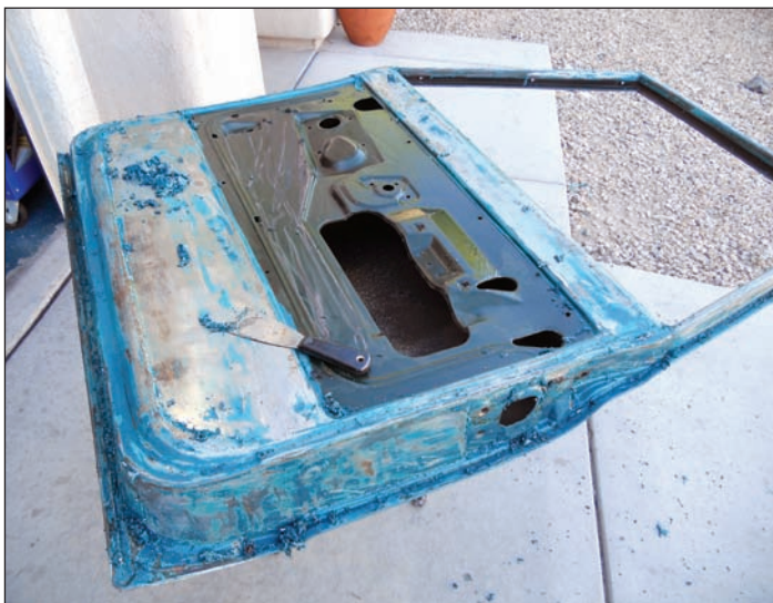
Aircraft stripper creates quite a mess, but it does get the job done for a relatively small amount of money. It needs a lot of elbow grease, but you will get a bare-metal finish once you're done if you do it correctly. (Photo Courtesy Mark Burdo)
