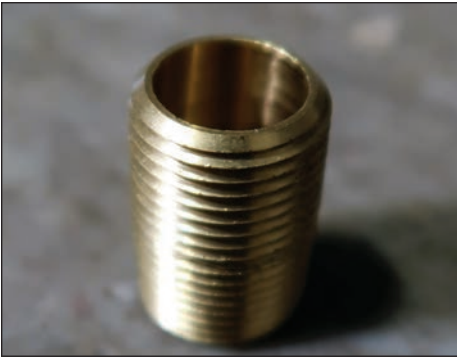
This is a straight NPT threaded cylinder, and it's called a close nipple. If you see the same thing with a wrench end in the middle, that is a hex nipple.
