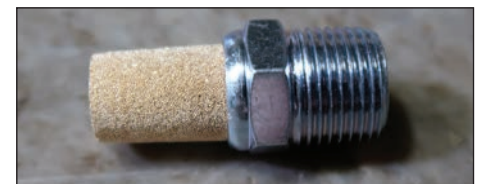
This is a weird-looking fitting. It's an NPT muffer, and it's designed to go into the end of a dump valve. This will slow down and quiet the air exiting the valve, which is nice if you want to either slow down your drops or tone down the noise.
