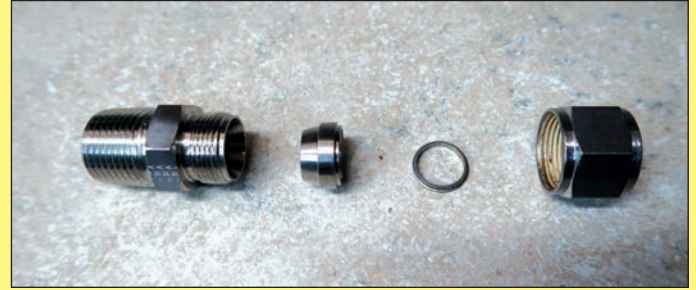
Inside each fitting are two compression sleeves. When used in the sequence shown, they can tighten down the line to the point that it'll be leak free.
