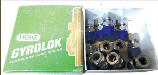
These Hoke Gyrolok fittings work just like Swageloks, but they're a bit more affordable.
