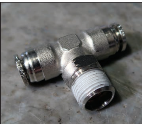
This is a branch T. If it was all the same end, it would just be a T-fitting, but the NPT base here makes it a branch T (If the NPT or dissimilar end was on one of the opposing ends of the T, it would be called a street T).
