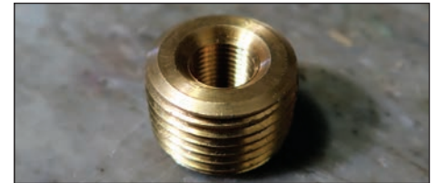
This is an NPT reducer bushing, which, in this case, is 1/2 to 1/8 inch. You'd use this if you wanted to put one end in a cross and run an 1/8-inch PTC fitting for an air gauge or something similar.
