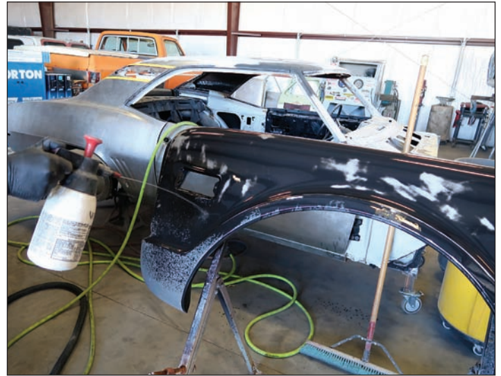
Back to the wax and grease remover we go with the entire panel getting another treatment of the cleaner. Just like before, he'll go over it with a lint-free paper towel, apply another round of cleaner, then paper towel a final time.
