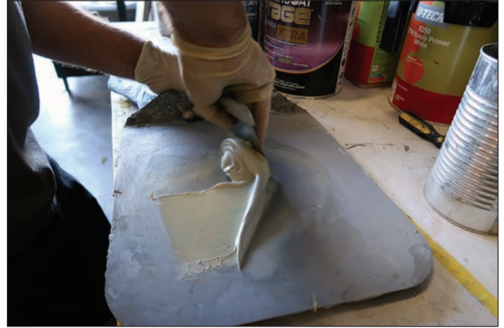
The hardener and the filler are mixed again, using pressing motions to push any air out of the material. The contrasting blue color should be thoroughly diffused in the filler before you move on to applying the product.
