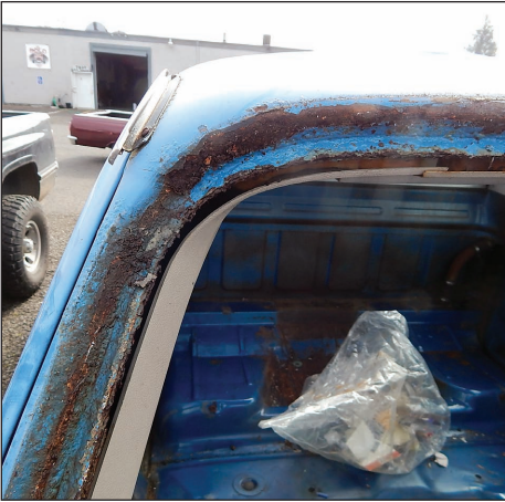
Many trucks of this era may have had a camper shell on them, and some of those have used a rubber gasket between the shell and the cab. If so, they may have a telltale rust line outside the normal boundaries of the rear window. (Photo Courtesy Lonnie Thompson)
