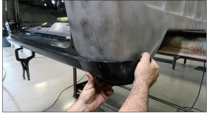
7 The replacement panel is fit back in place again, and now the tedious process of fitting, trimming, and fitting again begins. This will repeat itself until the panel fits perfectly on the body.
