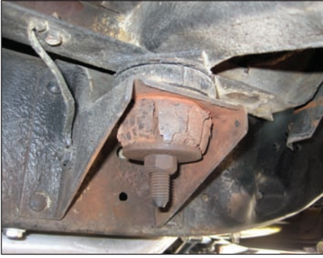
Rotten cab mounts look pretty rough, as evidenced by this pair. (Photo Courtesy Lee Hurlbutt)
