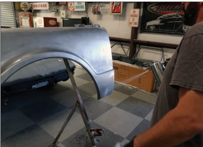
With the fender on a stand, the first step is to clean off the entire piece. In this case, it's wax and grease remover.
