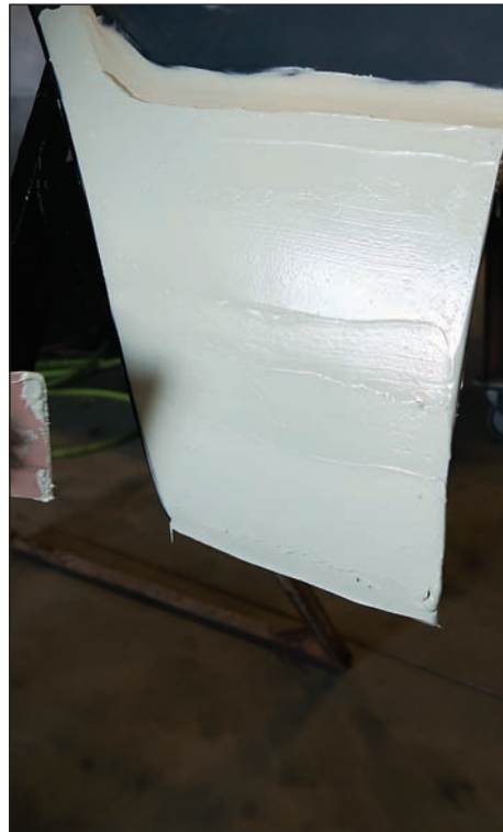
Once the filler is applied everywhere it needs to be, it's worked again, this time to smooth out any lines that were left vertically. What you're doing is making sure that everything gets sanded evenly instead of having mammoth peaks and valleys.
