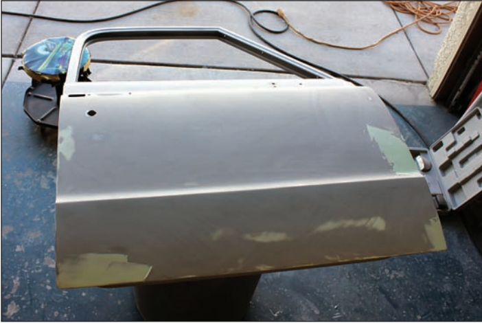
The filler is swiped on with a squeegee, and as you can see, it's kept as flat as possible but isn't perfect. That's fine; it'll get sanded down anyway. (Photo Courtesy Mark Burdo)
