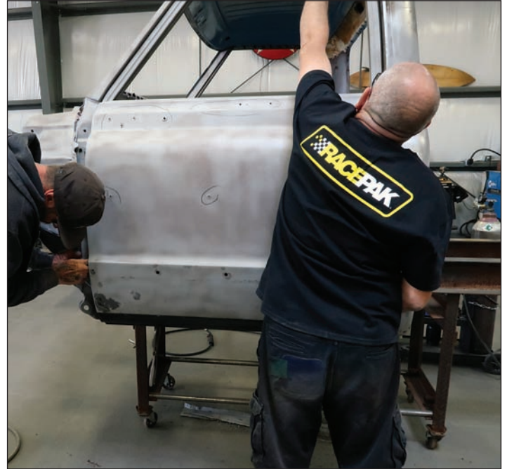
4 To make sure the rocker lines up correctly, the crew bolts up the original door to the body and gaps it properly.
