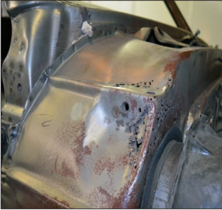
This truck, built in the Portland, Oregon, area, sported some repairable rust in the cowl. (Photo Courtesy Lonnie Thompson)
