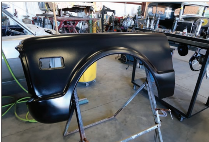
Once you have a part in bare metal, you have to cover it with something to prevent rust, right? In this case, yes—epoxy primer.
