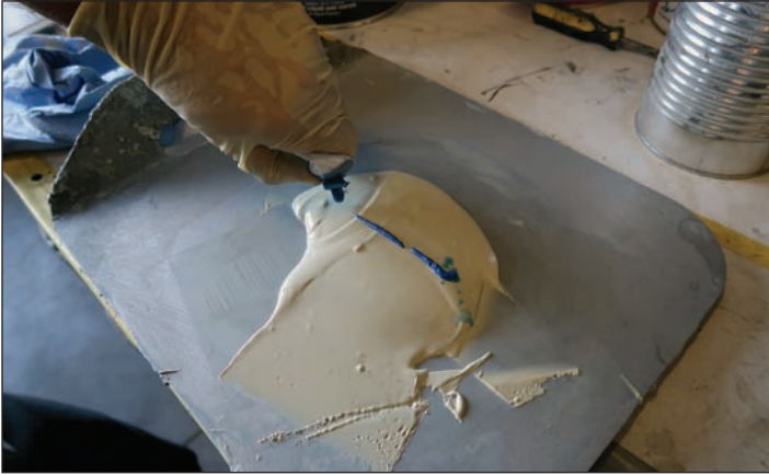
The hardener is put on next, and the general rule is to run a straight line of the product across the width of the filler. Hardener comes with every can of filler, but it's not inside the can. So if it's not handed to you at the paint counter, ask for it because you'll need it.
