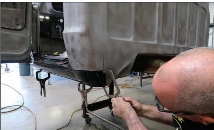
10 Now that the panel has been fitted correctly, Mike clamps it in place on the truck so that he can weld it in properly.
