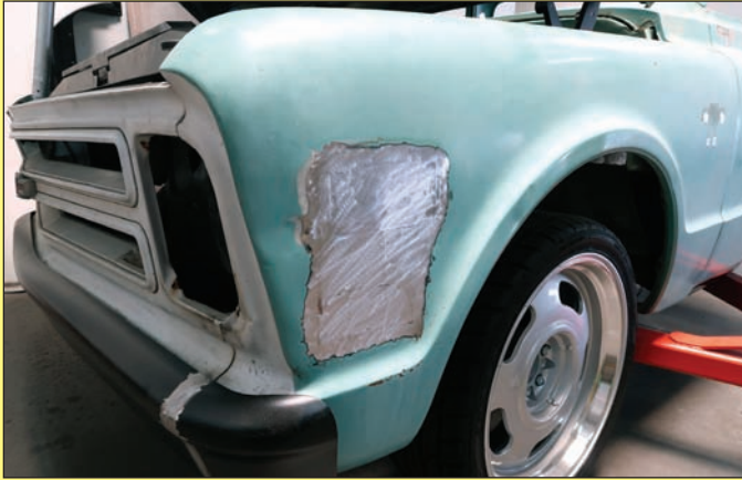
The stock sidemarkers on a 1968 C10 can be removed entirely from the fenders and bed and welded up, giving the truck the look of a 1967.
