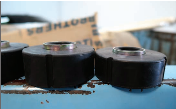
There are two different heights of cab mounts, and they're labeled when you buy replacements. Make sure you're putting the right ones in the correct places so you don't have alignment issues.
