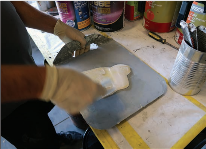
When you mix body filler, you want to be sure to work it consistently so as not to add bubbles into the material.
