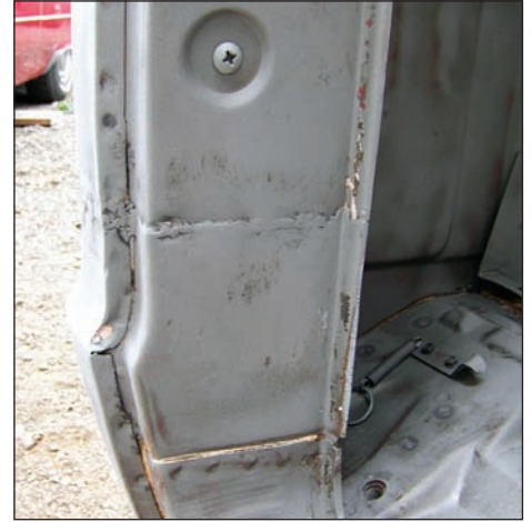
After blasting, you'll often find spots where previous repairs were performed. It's up to you to determine if they did a good job or not. (Photo Courtesy Lonnie Thompson)
