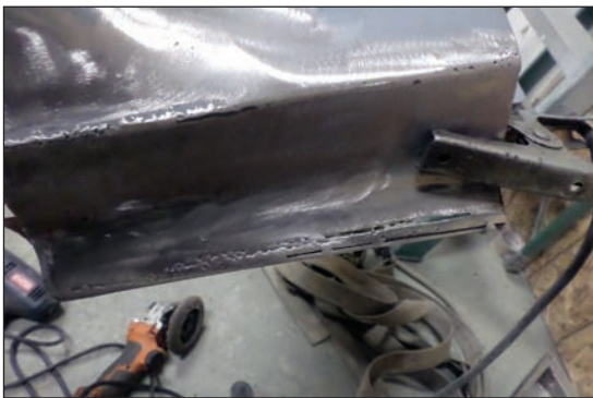
Here's a great example of panel gapping on a cowl. The factory piece didn't line up right, so they added some metal, then welded it all in place. (Photo Courtesy Lonnie Thompson)
