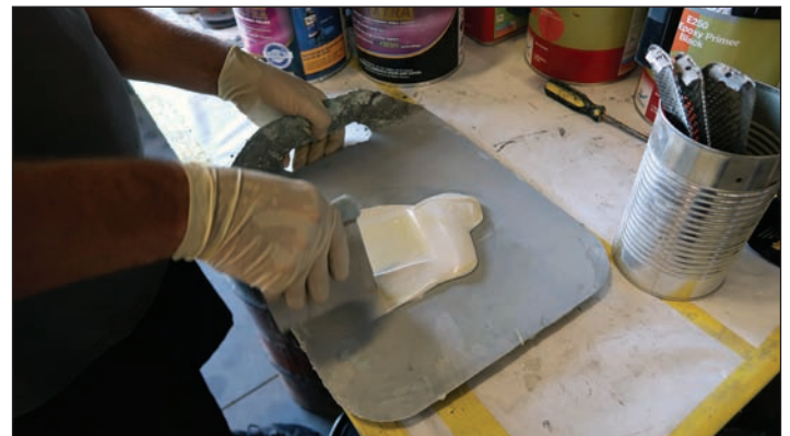
Now the two fillers are mixed together with a metal squeegee. This isn't done haphazardly; the two fillers are almost kneaded like bread dough, being sure not to push air into the process. It's tricky to do at first, but it gets much easier with practice.
