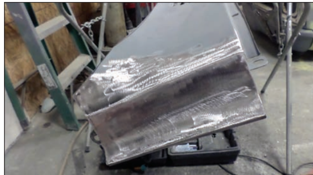
Once all the welding was done, it was ready for bodywork, so nobody would be the wiser. (Photo Courtesy Lonnie Thompson)
