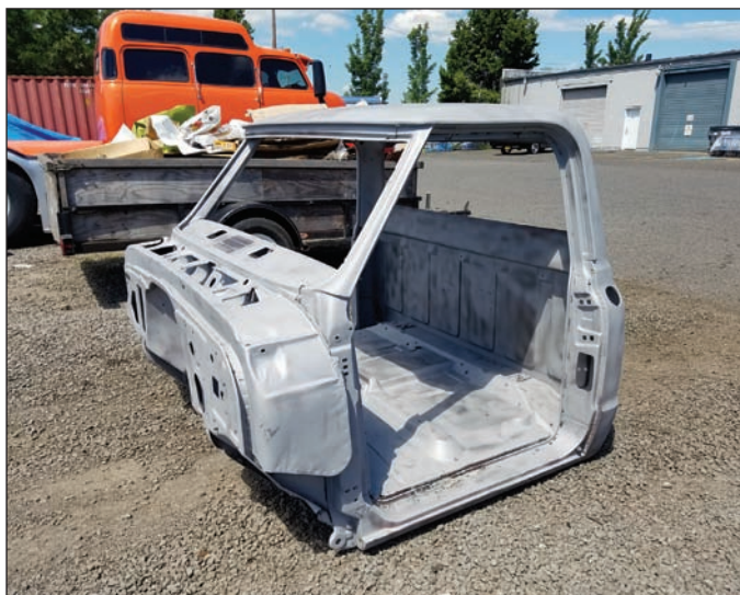
Here's a cab that just got back from the media blaster, and it's still in bare metal. (Photo Courtesy Lonnie Thompson)
