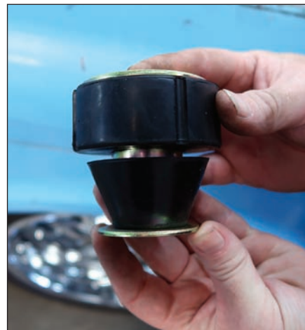
Removing the old cab mounts is pretty simple: unbolt them, jack up the side of the truck, and then lift them out. If you're concerned about damaging the rockers, use a block of wood between the jack and the panel to distribute the load.
