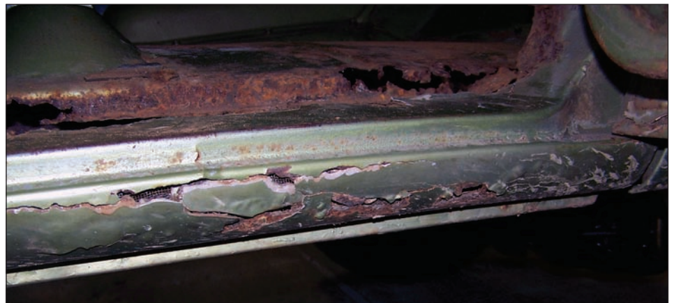
This is a great example of both a poor repair and severe rust. On the bottom of the rocker (and the corners where the floor meets the rockers) is severe rust that needs to be cut out. But above it is a previous repair job that involved fiberglass mat—not the proper application for this kind of job. (Photo Courtesy Lonnie Thompson)
