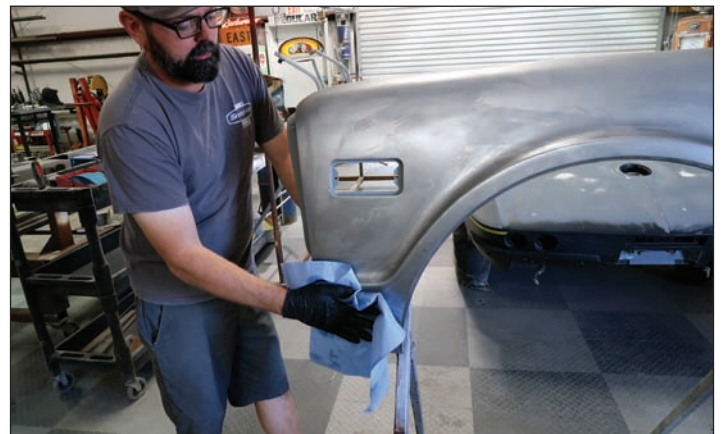
Using a clean, lint-free paper towel, the entire panel is then dried off. Notice that he's wearing gloves? That's to keep away from further contamination. This clean and dry process is done twice overall to ensure that everything is spotless.
