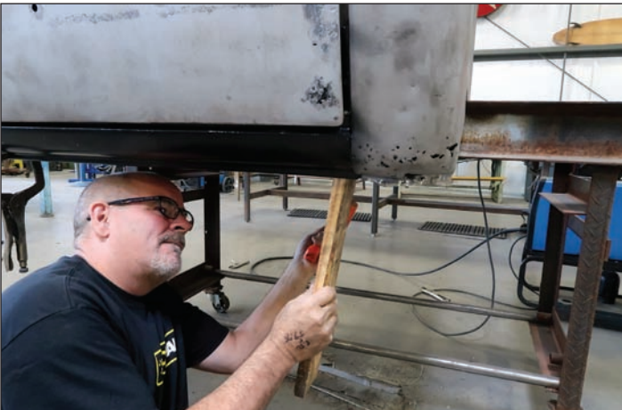
5 He starts by knocking the bottom of the rocker out farther using a block of wood to dissipate the blow from his hammer.
