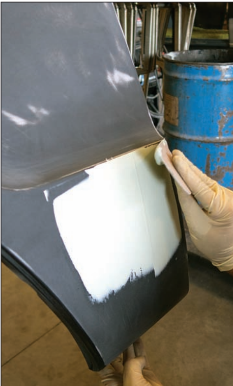
The filler is applied with a firm, consistent pressure from top to bottom. Again, the idea is to push out pinholes while still applying enough material. You want to go over the dent entirely, as well as beyond it by about 20 percent.
