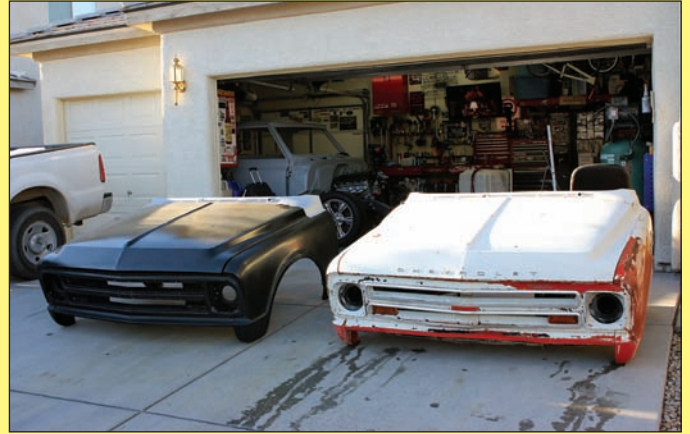
Here there are two 1967 front clips. In the foreground in white is one from a wrecking yard, and the one in black is made of aftermarket parts. (Photo Courtesy Mark Burdo)
