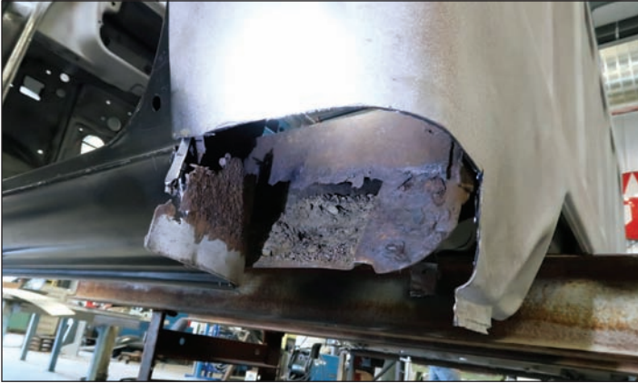
6 The inside of the panel is pretty rusted out too. It's covered in sand from the media blasting process, as well as rust.
