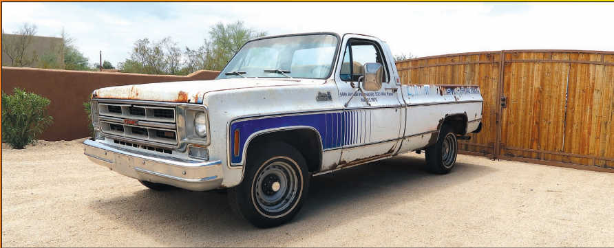
The truck, as it sits today, needs a bit of work. There's a ton of rust, particularly in the bed rails and bottoms of the fenders, but, surprisingly, the cab and cab floors are solid.
