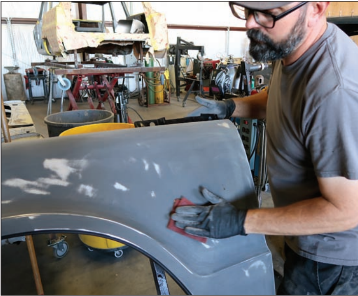
The entire panel is then lightly scuffed with a red Scotch-Brite pad. This is to hit any spots that may have been missed by the D/A, and it's done fairly quickly.
