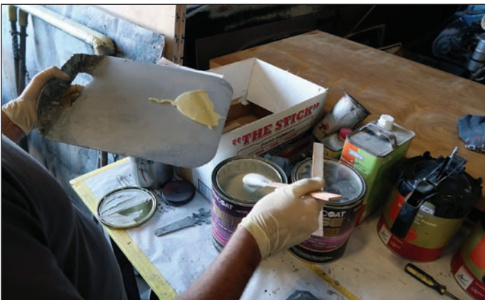
The idea here is to use a 50/50 mix of Rage Ultra and Rage Ultra Extra based on the temperature and work time needed. To do that, the raw filler is placed onto the mixing pad with a paint stick.
