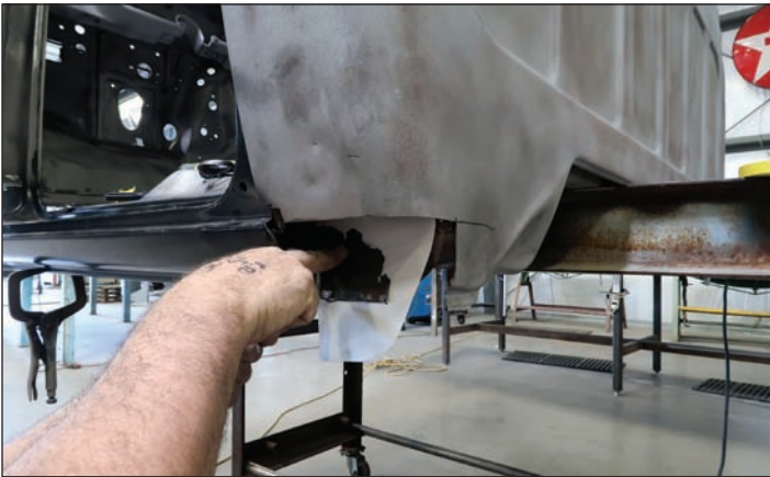
8 Using some poster board as a template, Mike marks out the area that he needs to replace. He'll use this as a guide on a piece of sheet metal so that it all fits like factory.
